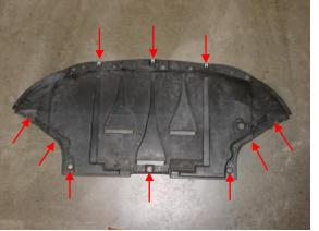
2. Remove diffuser by removing three (3) front, three (3) rear, two (2) left and two (2) right side fasteners.
