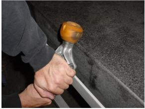
6. Separate isolator from torque arm by placing isolator on edge of stable surface and pull/push down to remove arm.
