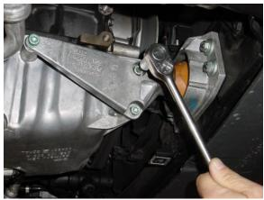
3. Remove three (3) bolts (6mm Hex driver) securing torque arm to oil sump.
