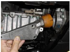
4. Remove torque arm from mount
