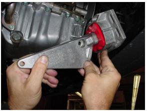
8. Install isolator into mount and re-position assembly for installation.
