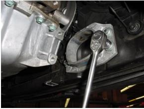
5. Remove three (3) nuts (13mm hex) securing mount to cross member and remove mount from vehicle.
