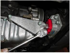
9. Install all fasteners by hand, then torque fasteners securing lever arm to oil sump to 20 Nm (15 ft-lb).
