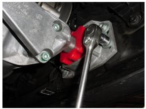
10. Position mount flush against cross-member and torque fasteners to 20 Nm (15 ft-lb).
