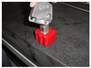
7. Place urethane isolator on stable surface and press torque arm into mount in orientation shown.
