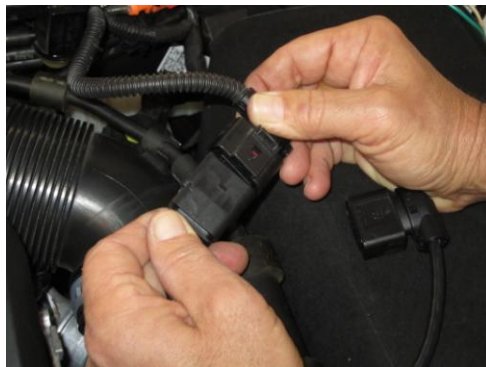
18. Connect vacuum line to port on NEUSPEED intake pipe.
