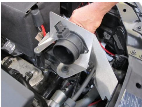
14. Install NEUSPEED P-Flo bracket onto rubber grommet mount and rubber isolator.
