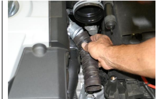
10. Remove hot air ducting hose.
