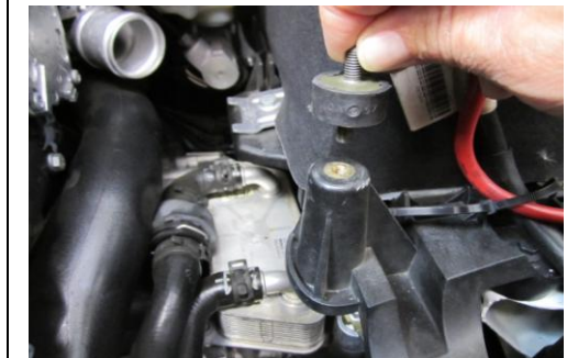
12. Install and tighten rubber isolator into threaded stand-off just in front of battery.
