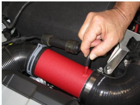
18. Connect vacuum line to port on NEUSPEED intake pipe.
