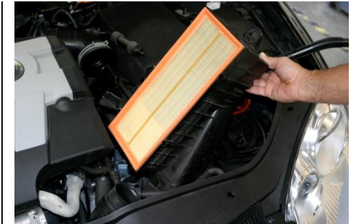
8. Lift off lower air filter box from rubber grommet mounts, then lift out left side first and rotate intake duct around small coolant hose to remove.
