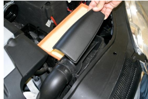
6. Remove cover at intake duct.
