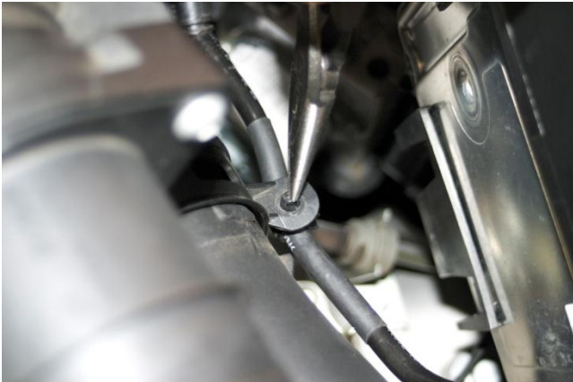
5. Separate brake booster line holder from fresh air intake hose. Use needle nose pliers to squeeze tabs and then push out holder.
