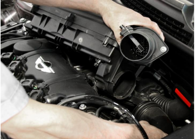
7. Locate fresh air pipe that is attached to air filter box. Disconnect fresh air pipe by rotating the 90° connection counter clockwise and pulling pipe away from air filter box. Remove air filter box from vehicle.
