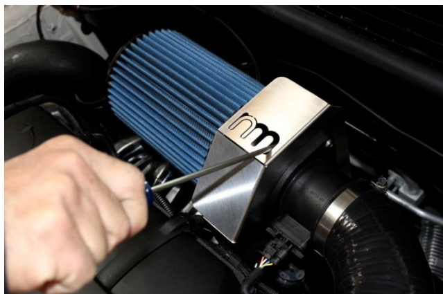
18. Using a degreaser or contact cleaner and shop rag, Clean inner mounting flange of NM filter. Install NM filter onto MAF sensor and tighten with long skinny screwdriver thru logo cut-out or from back side of bracket.
