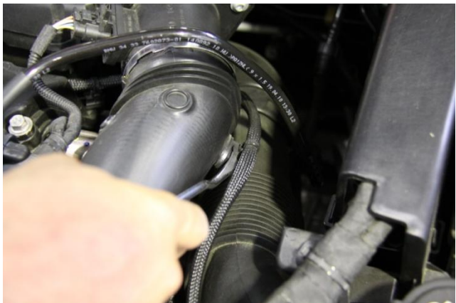
2. Remove the wire harness support mounts from the air intake tube.
