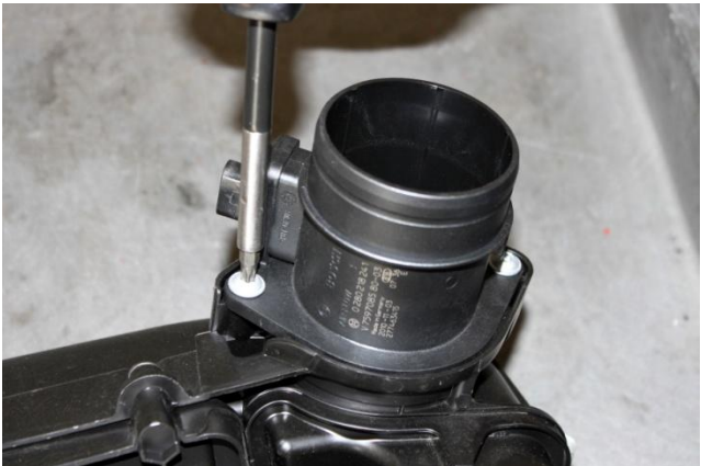
8. Remove MAF sensor from air filter box by removing [2] T30 TORX screws.
