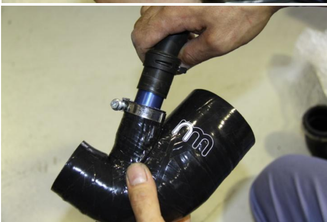
15. Remove factory breather hose from original air intake. Insert tube adapter (rolled lip end) into silicone turbo inlet hose and tighten with supplied #16 hose clamp. Connect breather hose onto tube adapter.
