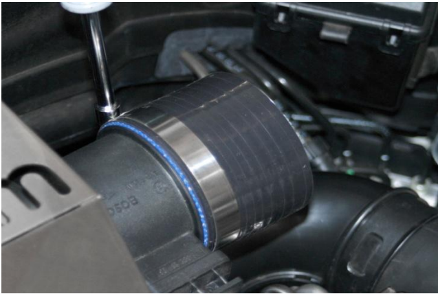
14. Install and tighten silicone coupler onto MAF sensor using supplied #44 hose clamp.
