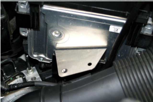
11. Remove protective film from double-sided tape on stainless steel fresh air hose bracket. Slide bracket down between ECU and black plastic ECU mount, while keeping double stick tape from touching. With bracket pushed all the way down, press against ECU.
