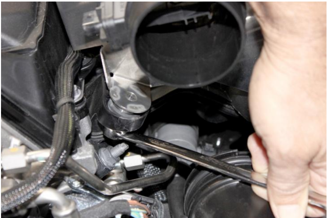
10. Install NM SS bracket onto factory air filter box mounts. NOTE: Make sure rubber grommets are still in place and not attached to bottom of the OE air filter box. From bottom side of mounts, install and tighten using supplied M8 washers and M8 lock nuts. [13mm socket and wrench]
