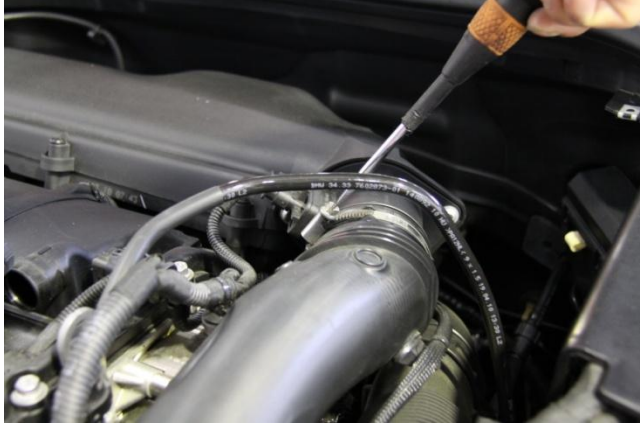
6. Remove T25 TORX screw located on passenger side of air filter box and lift off. NOTE: There are [3] pin mounts that are pushed into rubber grommet mounts on intake manifold, so effort may be required to lift air filter box off of mounts.
