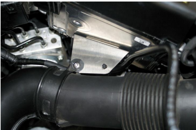
12. Attach brake booster line holder to forward mounting hole in bracket. Secure fresh air pipe to rearward mounting hole using supplied M6 x 10mm button head bolt. [4mm hex key wrench]
