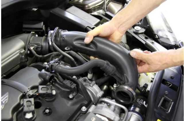
3. Use screwdriver to loosen clamps at turbo inlet and at MAF sensor. Remove air intake tube.
