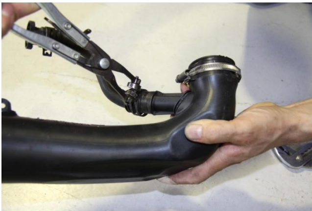
14. Install and tighten silicone coupler onto MAF sensor using supplied #44 hose clamp.
