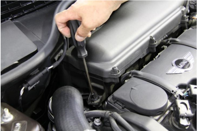
6. Remove T25 TORX screw located on passenger side of air filter box and lift off. NOTE: There are [3] pin mounts that are pushed into rubber grommet mounts on intake manifold, so effort may be required to lift air filter box off of mounts.
