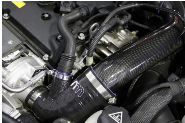
17. Loosely install supplied #44 clamps onto both silicone hose ends, then install air intake pipe into silicone turbo inlet hose first and then into MAF sensor hose. Adjust as necessary for clearance, paying close attention to clearance of silicone turbo inlet hose and coolant reservoir bottle. Tighten all clamps. NOTE: Do not forget to tighten #28 hose clamp from Step 16. Connect breather hose to cylinder head cover.
