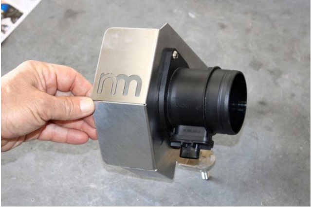
9. Install MAF sensor to NM stainless steel intake pipe bracket using supplied M6 x 16mm button head bolts and M6 nuts. [4mm hex key wrench / 10mm socket or wrench]
