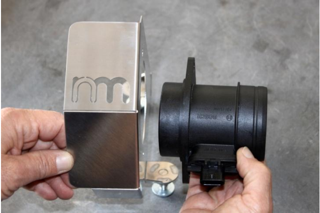
8. Remove MAF sensor from air filter box by removing [2] T30 TORX screws.
