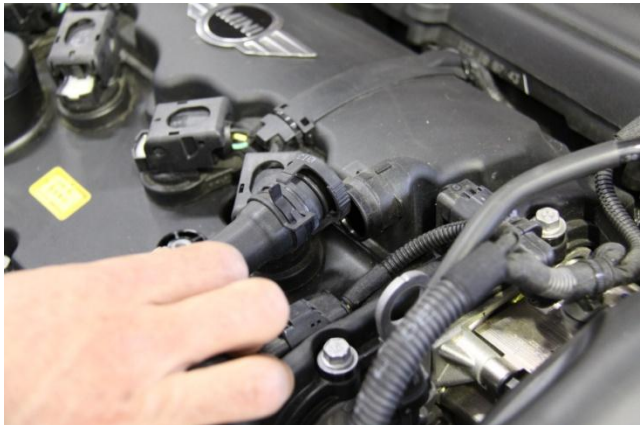
1. Squeeze the locking collar then pull-off breather hose to disconnect from cylinder head cover.
