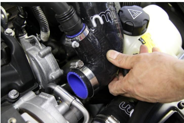
16. Loosely install silicone turbo inlet hose onto turbo using supplied #28 hose clamp. NOTE: Do NOT tighten at this time.
