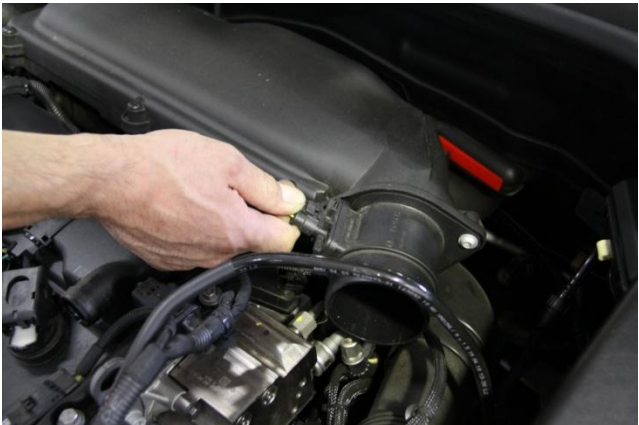
4. Squeeze locking tab then disconnect electrical connector from Mass Airflow Sensor (MAF).
