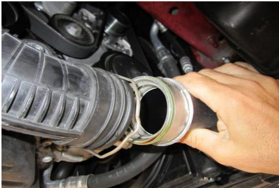
3. Pull-out clip to release rubber intercooler hose from turbo discharge plastic pipe.
