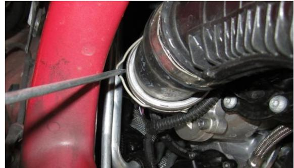
5. Pull-out clip to release upper rubber hose from turbo, and then remove turbo discharge pipe.
