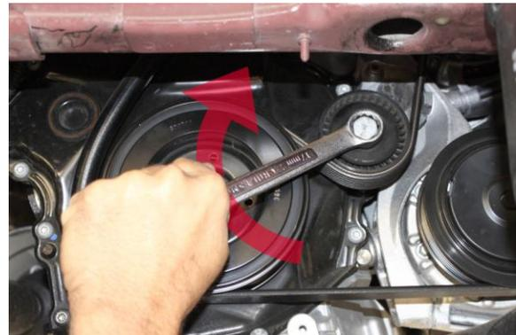
8. Using a 17mm wrench, rotate idler pulley center bolt upwards to release tension and remove ribbed belt. Now slowly release belt tensioner.
