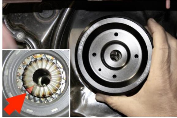
11. Use a little oil on timing cover seal. Install *NEUSPEED* pulley matching up tooth contour on pulley with crankshaft chain sprocket, while holding against chain sprocket install new bolt supplied and hand tighten.
