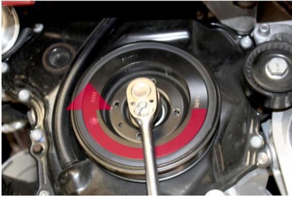
9. Using the 24mm socket on crankshaft pulley bolt, rotate engine clockwise to the "TDC" position (Top Dead Center). The notch on the pulley must line-up with the arrow marking on the timing chain cover located on top of the side of the pulley.
