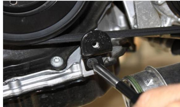
6. Remove discharge pipe mounting bracket from engine using T30 Torx.
