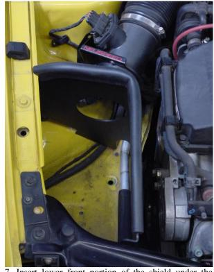
7. Insert lower front portion of the shield under the radiator support and slide bottom edge of shield into slot between AC condenser line and chassis seam. Rotate rear portion of shield down and into position, making sure any hoses and/or electrical lines are routed through cut outs.
