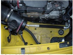
6. Re-install intake hose to mass air sensor and reconnect electrical connector. At this point, your installation should like what is pictured above.
