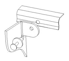
8. Due to slight variations in vehicle geometry (see illustration above), it is necessary to drill the front mounting tab and radiator support to properly mount the heat shield. Pull the heat shield forward (towards the front of the car) until the mounting tab contacts the radiator support. Determine hole location on center of radiator support and transfer that location to front mounting tab. Remove heat shield and drill  $\emptyset$  ½" hole through tab.
