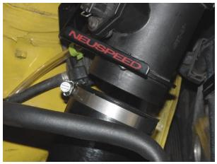
11. Pass newly supplied filter through opening in heat shield. Rotate filter until end of filter is parallel with mass air sensor. Slide filter onto sensor and secure hose clamp. NOTE: Check tightness of clamp in one week.
