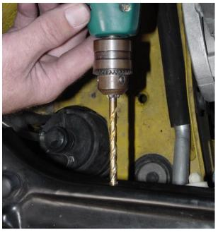
9. Install heat shield and using the front mounting tab hole as a guide, mark the radiator support. Remove the shield and drill a  $\varnothing$   $\frac{1}{4}$ " hole through the radiator support.
