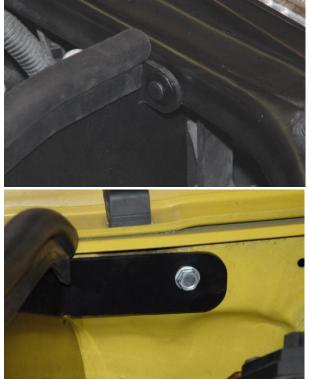
10. Install the heat shield and secure in front with the supplied push fastener and at the side with the supplied sheet metal screw as shown.
