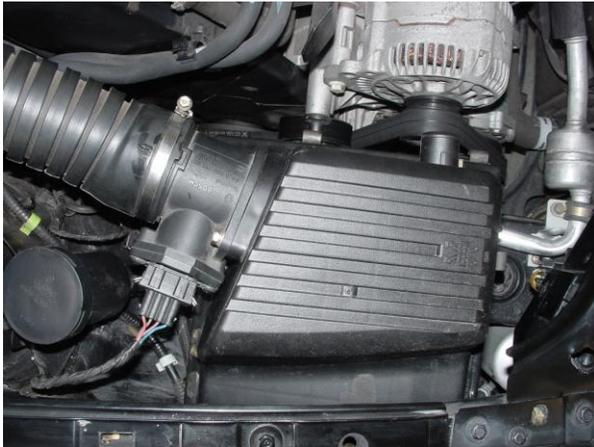
1. First, disconnect mass air sensor from air box. Next, unclip upper filter housing, remove air pump hose and disconnect small vacuum line from manifold port. Cap port with supplied plug and remove filter housing top. Remove hot air tube between lower filter housing and exhaust heat shield. Remove rubber ‘O’ rings that hold air box to frame and remove lower filter housing.
