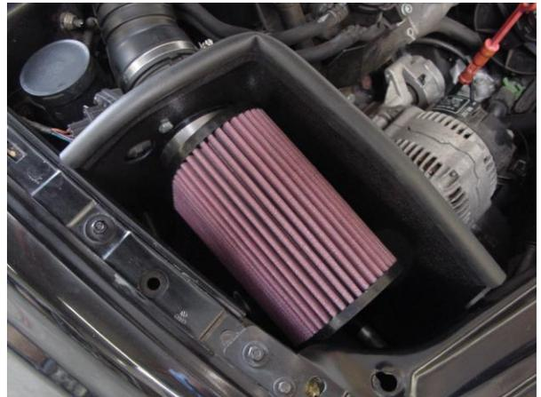
7. Mount mass air sensor to heat shield using supplied 1/4" bolts and lock nuts. Install air filter on mass air sensor and tighten hose clamp. **NOTE: Check tightness of clamp in one week.**
