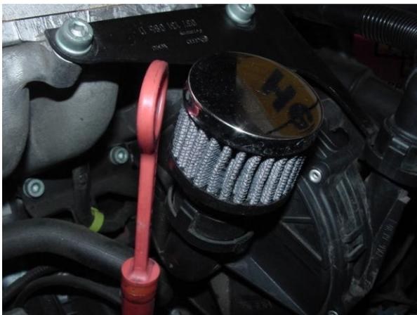
2. Install mini-filter to air pump, if equipped.
