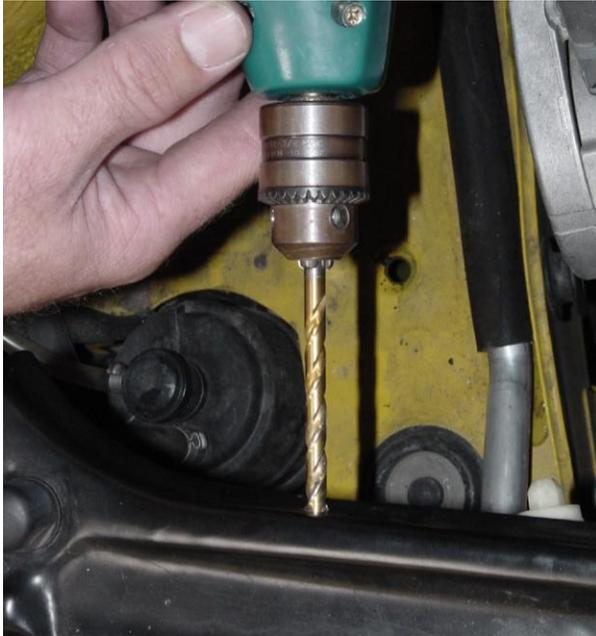
5. Remove the head shield and drill a  $\varnothing$  1/4" hole through the radiator support.
