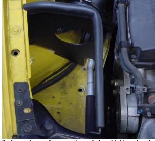
3. Insert lower front portion of the shield under the radiator support and slide bottom edge of shield into slot between AC condenser line and chassis seam. Rotate rear portion of shield down and into position, making sure any hoses and/or electrical lines are routed through cut outs.
