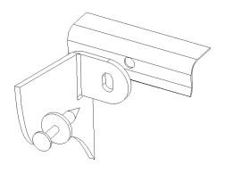
4. Due to slight variations in vehicle geometry (see illustration above), it is necessary to drill the radiator support to properly mount the heat shield. Pull the heat shield forward (towards the front of the car) until the mounting tab contacts the radiator support. Using the front mounting tab hole (slotted) as a guide, mark and center punch the radiator support.
