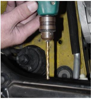
5. Remove the head shield and drill a  $\emptyset$   $\frac{1}{4}$ " hole through the radiator support.
