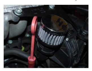
2. Install mini-filter to air pump, if equipped.
