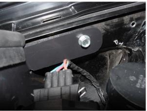
6. Install the heat shield and secure in front with the supplied push fastener and at the side with the supplied sheet metal screw as shown.
