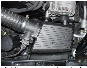
1. First, disconnect mass air sensor from air box. Next, unclip upper filter housing, remove air pump hose and disconnect small vacuum line from manifold port. Cap port with supplied plug and remove filter housing top. Remove hot air tube between lower filter housing and exhaust heat shield. Remove rubber 'O' rings that hold air box to frame and remove lower filter housing.
