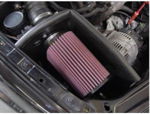
7. Mount mass air sensor to heat shield using supplied 1/4" bolts and lock nuts. Install air filter on mass air sensor and tighten hose clamp. **NOTE: Check tightness of clamp in one week**.
