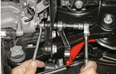
Using supplied M10 x 65mm bolt, install thru NEUSPEED end-link, then stainless steel spacer with taper toward spherical bearing, then through trailing arm. Secure with original locknut and torque to 40Nm (30 ft-lb). NOTE: Passenger side shown.
