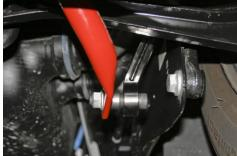
Reinstall wheels, lower vehicle and torque wheel bolts to manufacturer's specifications. NOTE: With suspension unloaded, spherical bearing will be at maximum angle. Once suspension is loaded, end-link and spherical bearing will self-align into position as shown in photo.
