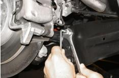
Remove both rear wheels. Remove both rear end-links from trailing arm and anti-roll bar by securing stud with M6 triple square or 5mm hex key wrench, while loosening nut with 16mm wrench.
