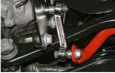
Using supplied M10 x 50mm bolt install thru NEUSPEED end-link, then stainless spacer with taper towards spherical ball, then through anti-roll bar. Secure with original locknut and torque to 40Nm (30 ft-lb). NOTE: Passenger side shown.
