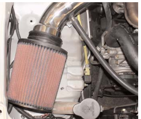
Once the filter has been placed over the intake end and the intake is set up against the filter stop continue to tighten the filter clamp.
