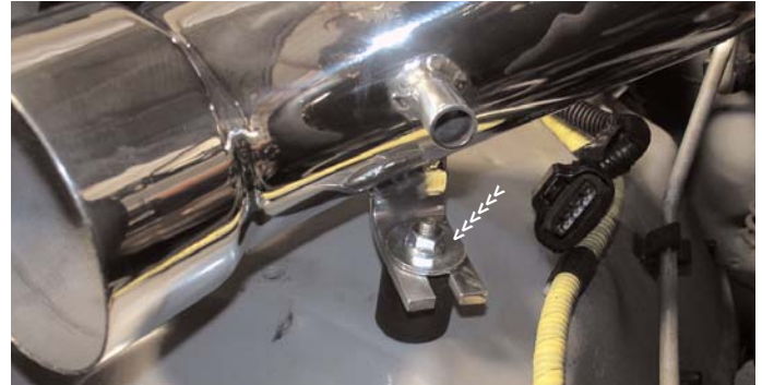
The flange nut and fender washer is screwed onto the vibra-mount stud. Do not over-tighten the flange nut at this point until the filter has been placed on the end.
