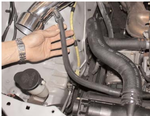
The 14"- 10mm vacuum hose is now pressed over the 1/2" intake port as shown above.
