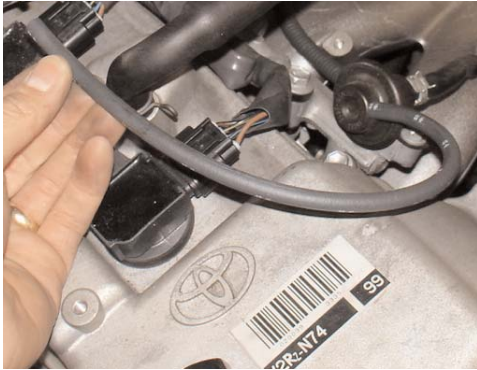
The stock 4mm hose remains on the pressure fuel regulator.
