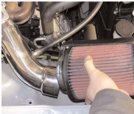
The 3 1/2" inverted top filter is set in the engine compartment ready to be installed.
