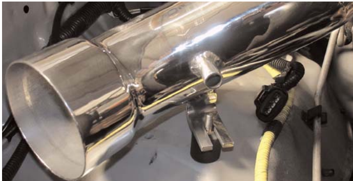
The intake bracket is sitting flush over the vibra-mount stud and lined up to the throttle body.
