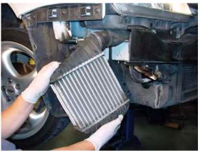
3. Remove factory intercooler: Unclip and remove air ducting from intercooler. Disconnect boost sensor wire harness from sensor at top intercooler end-tank. Remove (2) 10mm hex bolts at top of intercooler and (1) 10mm hex bolt at bottom of intercooler. Disconnect inlet hose at bottom of intercooler and upper hose at throttle body. Unclip wire loom from rubber intake hose. Carefully, remove factory intercooler and attached intake hose.
