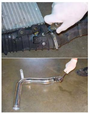
14. Remove (2) Phillips screws from factory boost sensor. Remove boost sensor from factory intercooler. Install aluminum boost sensor adapter onto fitting on L-shaped tube. Then install boost sensor onto fitting as shown. Fasten with (2) M6x20mm socket head bolts (supplied). **NOTE: Use caution when tightening – do not over tighten.** Install L-shaped tube from bottom side of vehicle.
