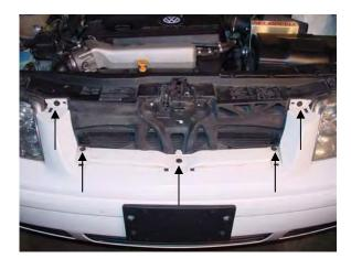
2a. Remove bumper cover: On top remove the (5) Torx T30 screws.
