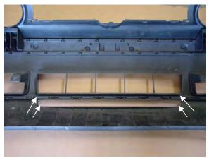
22a. Re-install bumper cover <u>Golf</u>: Trim backside of bumper cover as indicated by arrows. Start at corners of grill openings and feather trimming outwards. Double-check clearance and proceed to step 23.
