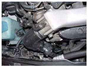
16. Connect upper end of L-shaped tube to throttle body with  $90^{\circ}$  silicone elbow with (1) supplied hose clamp to intercooler tube. Re-use OE throttle body hose clamp at throttle body. Do not tighten hose clamps at this time.
