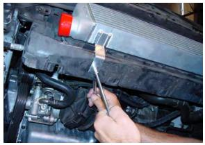
11. Use (2) M6x20mm bolts, (2) washers, and (2) nyloc nuts to fasten intercooler to lower radiator core.
