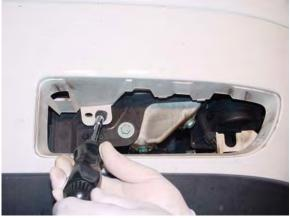
2b. Up front, remove both outer grill inserts by pushing down release tabs at top corners. Remove (1) Torx T30 screw from each side.
