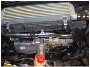
18. Use <sup>1</sup>/<sub>4</sub>" drill bit and drill hole for U-bent tube mounting bracket. **NOTE: Mind drilling depth to be careful not to puncture radiator.** Mount U-bent tube with M6 x 20mm hex bolt, washer, and nyloc nut. Tighten all hose clamps at this time. Double-check clearances. Re-connect boost sensor wire harness – position wires loom away from fan and drive pulleys.
