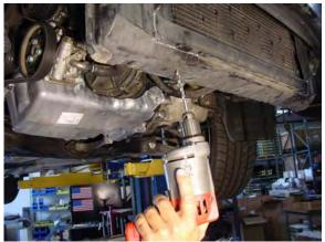
9. Using <sup>1</sup>/<sub>4</sub>" drill bit, drill marked holes. **NOTE:** Mind drilling depth to be careful not to puncture radiator.
