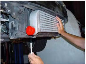
8. Position intercooler core with brackets inside of cut grooves and with upper channels pushed up against bottom lip of metal bumper structure. With marking pen, mark position of holes through mounting brackets.
