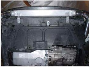
21. Re-install center under tray. Trim leading edge of under tray for proper clearance of intercooler and intercooler tube mounting brackets.
