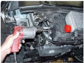
17. Center L-shaped tube between A/C receiver drier and power steering pulley for best clearance and mark hole for bracket mounting. **NOTE: If you plan on using our Power Pulley kit in the future, you will need to space L-Shaped pipe closer toward A/C receiver drier**. Use <sup>1</sup>/<sub>4</sub>" drill bit and drill hole. **NOTE: Mind drilling depth to be careful not to puncture radiator.** Mount L-shaped tube with rubber isolator mount, washer, and M6 hex nuts.
