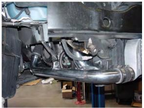
19. Install intercooler inlet pipe to factory turbo hose and to intercooler inlet end-tank. On end-tank side, remove protective cap from inlet side of intercooler end-tank and use a straight siliconee hose and two hose clamps. Screw drive of clamps should be on top side as shown. Use original intercooler mounting bolt to fasten intercooler inlet pipe to original bracket. Tighten hose clamps at this time.
