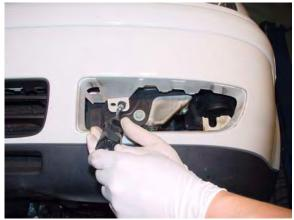
23. Use spacers (supplied) behind bumper cover lower mounting tabs. Re-install bumper cover in reverse of disassembly.
