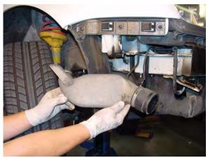
4. Remove OE pancake pipe by removing (1) 10mm hex nut and loosening hose clamp.
