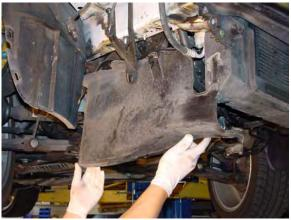
6. Remove two lower side engine covers by removing (1) Torx T25 screw and unscrewing (2) metal retaining clips on each cover. **\(\Cov\_Hint:** Use flat head screw driver to rotate metal retaining clip counter-clockwise. Passenger-side shown.
