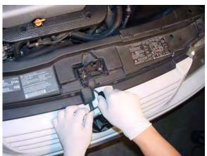
1. Remove factory grill by prying up metal retaining clip of hood release lever. Using a screw driver spread the plastic release lever open to disconnect from hood latch. Release grill attachment clip located in square hole on top of grill by pushing down plastic catch with screw driver. Disconnect upper corners of grill by pulling forward. Tip grill forward and pull up to release grill.
