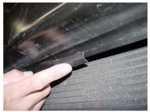
10. Attach foam tape (supplied) around lip of steel bumper structure where intercooler channel will be inserted.
