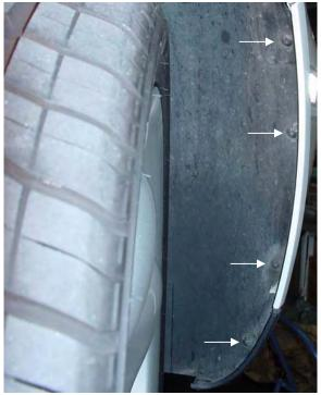
2c. In each fender well, remove (4) Torx T25 screws. Pull bumper cover forward at each corner and disconnect side marker lamp harness from each side. Remove bumper cover.
