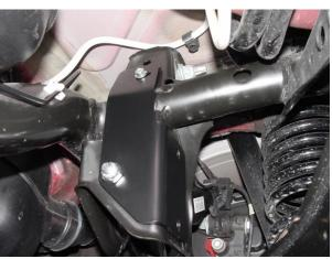
5. Loosely mount Left and Right Support Brackets, do not tighten at this time. Now follow *NEUSPEED* Anti-Roll Bar installation instructions. **NOTE**: Evenly tighten Anti-Roll Bar bushing clamp bolts and Support Bracket bolts.
