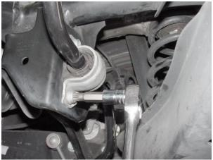
2. Remove the (4) anti-roll bar bushing clamp mounting bolts using a M10 Triple Square or 8mm hex key wrench.
