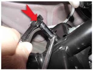
4. Installing Nutsert, hold tool body with 9/16" wrench from turning and push down on Ratchet while crimping Nutsert into hole.
