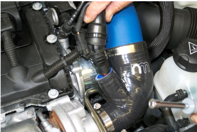
16. Install valve cover breather into silicone turbo inlet hose.
