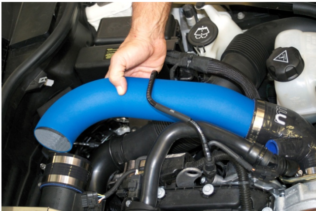
15. Loosely install supplied #44 clamps onto both silicone hose ends, then install aluminum intake pipe into silicone turbo inlet hose first and then into MAF sensor hose. Adjust as necessary for clearance, paying close attention to clearance of silicone turbo inlet hose and coolant reservoir bottle. Tighten all clamps. NOTE: Do not forget to tighten #28 hose clamp from Step 14.
