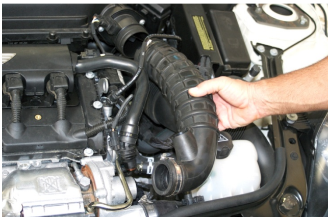
2. Remove OE turbo inlet hose from MAF sensor. Use screwdriver to loosen clamp at turbo inlet and at MAF sensor.
