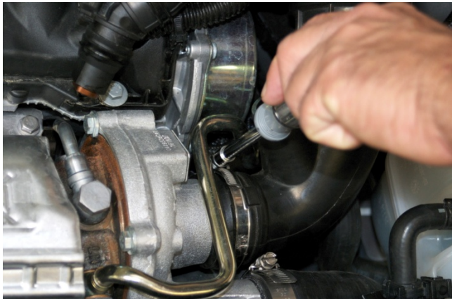
1. Pull out valve cover breather hose from OE turbo inlet hose.
