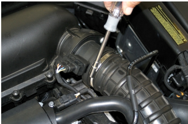
5. Remove T25 TORX screw located on passenger side of air filter box and lift off. NOTE: There are [3] pin mounts that are pushed into rubber grommet mounts on intake manifold, so effort may be required to lift air filter box off of mounts.
