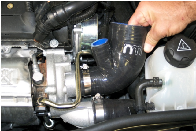
14. Loosely install silicone turbo inlet hose onto turbo using supplied #28 hose clamp. NOTE: Do NOT tighten at this time.
