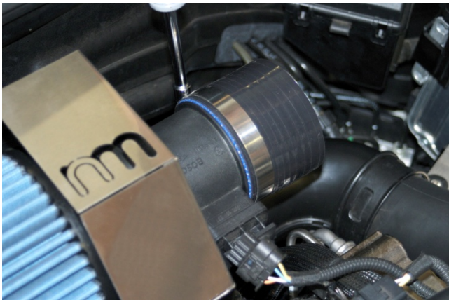
13. Install and tighten silicone coupler onto MAF sensor using supplied #44 hose clamp.
