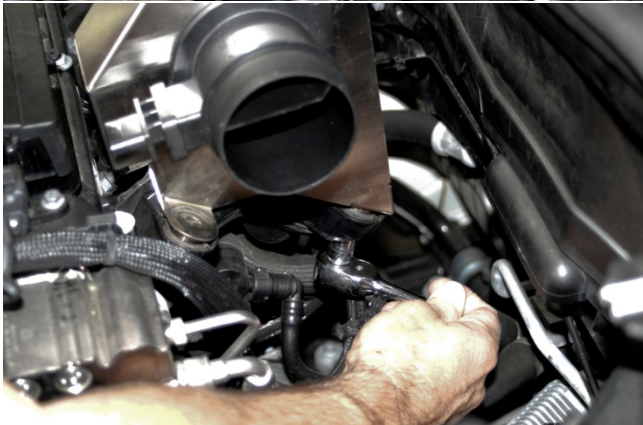
10. Install NM filter assembly unit onto factory air filter box mounts. NOTE: Make sure rubber grommets are still in place and not attached to bottom of the OE air filter box. From bottom side of mounts, install and tighten using supplied M8 washers and M8 lock nuts. [13mm socket or wrench]
