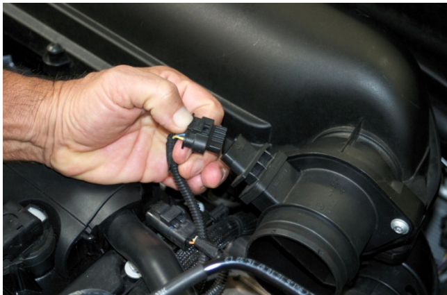
3. Disconnect electrical connector from Mass Airflow Sensor (MAF).
