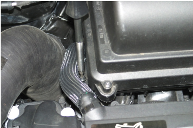
5. Remove T25 TORX screw located on passenger side of air filter box and lift off. NOTE: There are [3] pin mounts that are pushed into rubber grommet mounts on intake manifold, so effort may be required to lift air filter box off of mounts.
