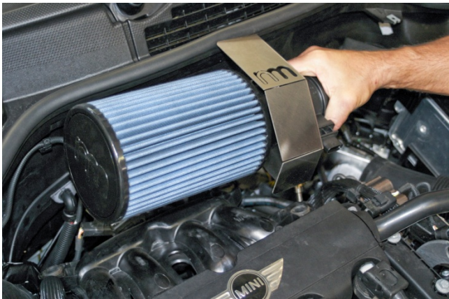
9. Using degreaser or contact cleaner and shop rag, clean inner mounting flange of NM filter. Install and tighten filter onto MAF sensor. Position NM logo on end of filter for proper reading orientation.
