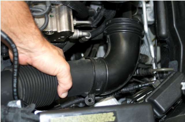
6. Locate fresh air pipe that is attached to air filter box. Disconnect fresh air pipe by rotating the 90° connection counter clockwise and pulling pipe away from air filter box. Remove air filter box from vehicle.
