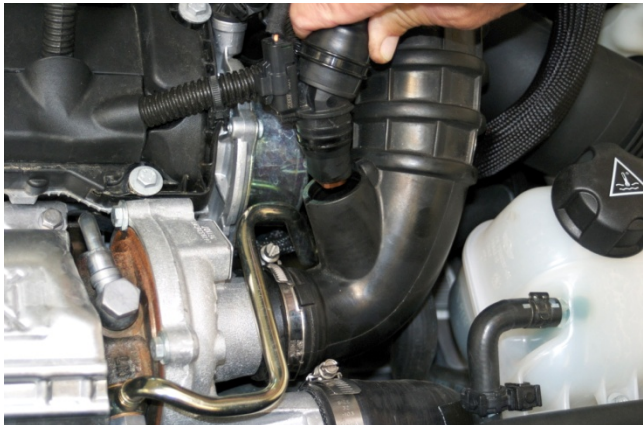
1. Pull out valve cover breather hose from OE turbo inlet hose.
