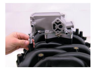
Once the spacer is in place, using factory torque specifications, you may tighten the 4 bolts on the flange of the upper intake manifold. Once the four bolts are tightened you may tighten the final bolt on the support leg to the specified torque value.
