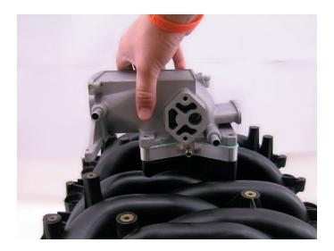
Now install the 4 main intake bolts to secure the upper manifold and nitrous plate to the lower plastic intake manifold. Do not tighten.
