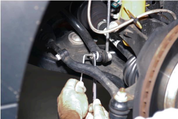
4. Unbolt nut from anti-sway bar to end link using a 16mm wrench and 5mm hex key wrench. Repeat for other side. NOTE: To ease removal spray threads with WD-40 and then break nuts loose first using a 16mm socket.
