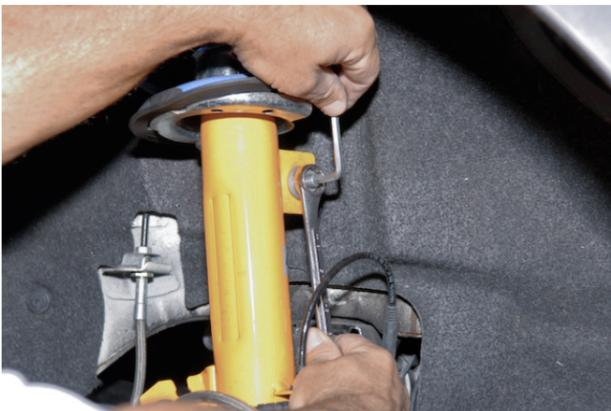
5. Unbolt end link from strut mount using a 16mm wrench and a 5mm hex key wrench, then remove end link. Repeat for other side.
