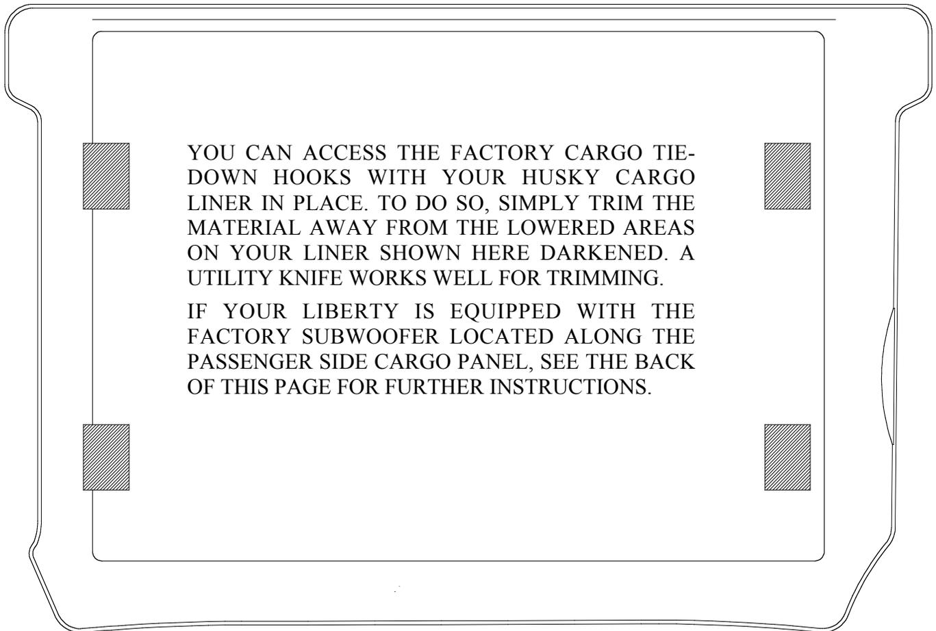
LIBERTY CARGO LINER SHOWN TRIMMED FOR OPTIONAL FACTORY SUBWOOFER. TO TRIM FOR THIS OPTION, SIMPLY REMOVE THE MATERIAL FROM THE RECESSED AREA MOLDED INTO THE LINER. USE THE EDGE OF THE RECESSED ARC AS YOUR TRIMMING GUIDE.
