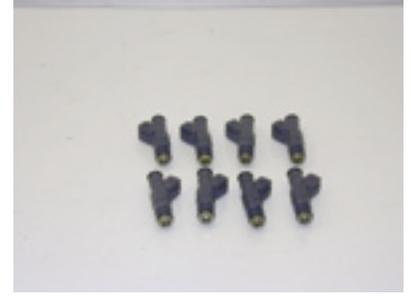
5. Flip injector rail over. This will allow you to remove injector lock clips. Once you have removed the clips take the injectors off of the fuel rail. Then inspect both o-rings on every injector. If the o-ring has the slightest tear or cut, replace before reinstalling.
