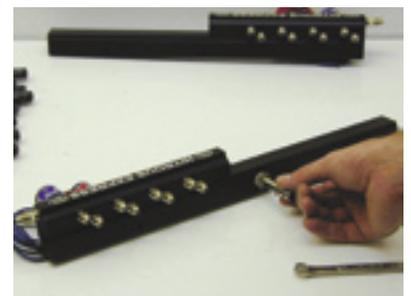
6. The rail fittings are installed in house. Then the rails are pressure checked to ensure a proper seal. The fuel fitting must be installed next. It is located on the drivers side rail directly in the center. As with all pipe-thread fittings you must use NX thread sealer on all threads.
