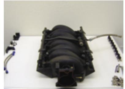
2. Use a slip-lock disconnection tool to remove your fuel line. Just disconnect the line and pull off of your fuel rail
