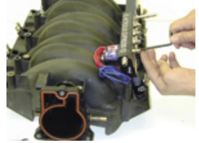
8. Once you have completed all of the before steps, it is now time to install the NXL rail. Just gently place the rail and injectors over the NXL nozzles and line them up. Press evenly and firmly until all injectors are fully seated in the nozzles. Then screw in the allen head screws through the fuel rail bracket and into the NXL fuel rail. You may finish tightening the rail mounting studs on the intake.
