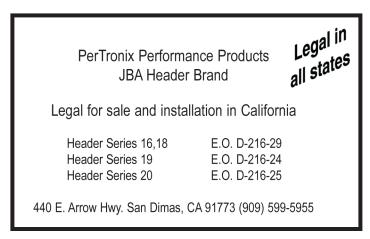
This sticker is required to aid in passing the California Smog Check Program. This sticker must be installed in an underhood location that is readily visiblle.
