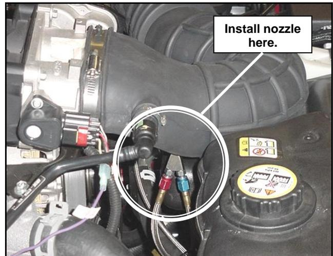
Figure 5 Soft Plume Nozzle Installation Cut-Away & Installation Photo
