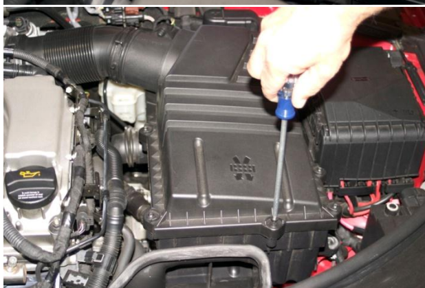
4. Unbolt left front corner of lower air box using 5mm hex key wrench. Lift off lower air box from two rubber mounting grommets and remove from vehicle.
