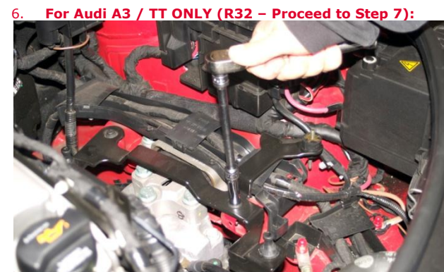
a. Using 10mm socket, remove front bolt on air box mounting bracket.
