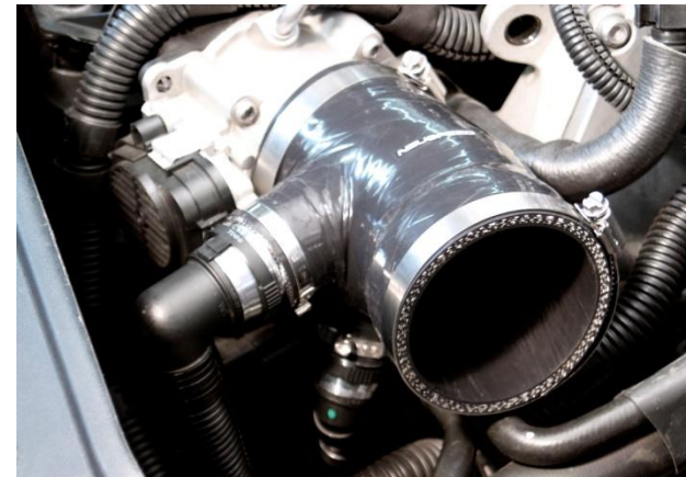
7. Connect crankcase ventilation hose and Secondary Air Injection hose to billet fittings on silicone hose. NOTE: For vehicles not equipped with Secondary Air Injection use supplied vinyl cap and wire tie on billet fitting.
