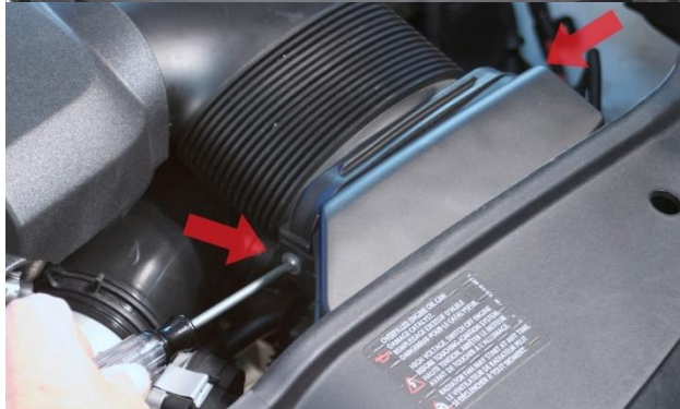
1. Remove (2) T20 Torx screws from air intake duct.
