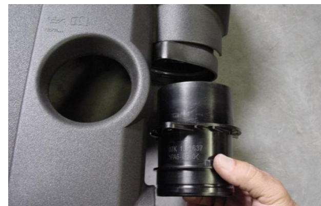
8. Remove (2) Phillips screws that mount the air box inlet adapter to engine cover and separate.
