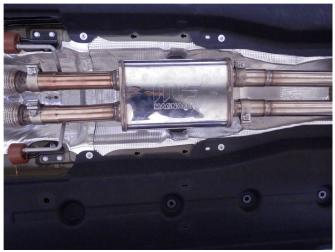
**Step 2.** Begin installation of the new system by loosely attaching the Resonator Assembly to the outlets using the 2.25" clamps. Leave all clamps loose until final adjustment.
