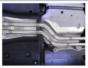
**Step 3.** Next attach the Mid Pipes to the Resonator Assembly using the supplied 2.25" clamps.
