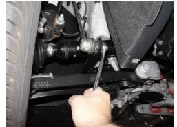
i. Unbolt anti-roll bar from end-links 18mm hex nut.
