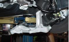
7. Unbolt aluminum control arm mount from uni-body and let swing down. NOTE: Because of enlarged mounting holes, use marking pen to mark location of control arm mount to uni-body. This will aid in keeping the original alignment.
