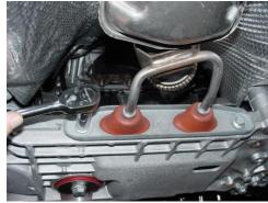
Unbolt torque arm from transmission housing (2) 16mm hex bolts and exhaust down-pipe support bracket from rear of aluminum sub-frame (2) 13mm hex bolts.
