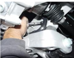
Driver's side of vehicle: Unbolt plastic wire guide from aluminum control arm mount 10mm bex bolt.
