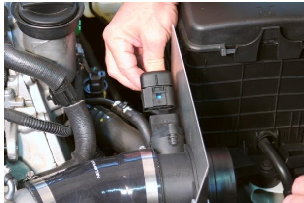
16. Plug MAF wire connector into MAF.
