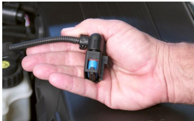
15. Install new supplied shield with wires facing down.
