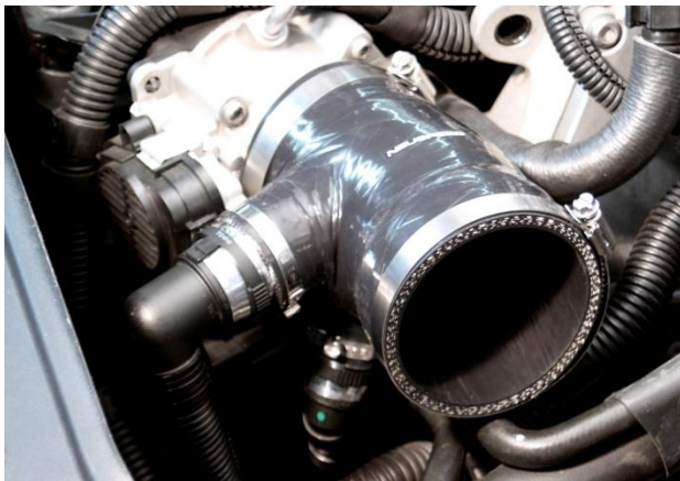
9. Connect crankcase ventilation hose and secondary air injection hose to billet fitting on silicone hose.
