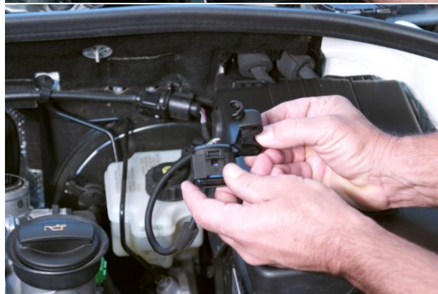
14. Unclip and remove MAF wire connector shield.
