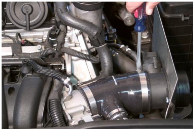
13. Tighten both silicone hose clamps now.
