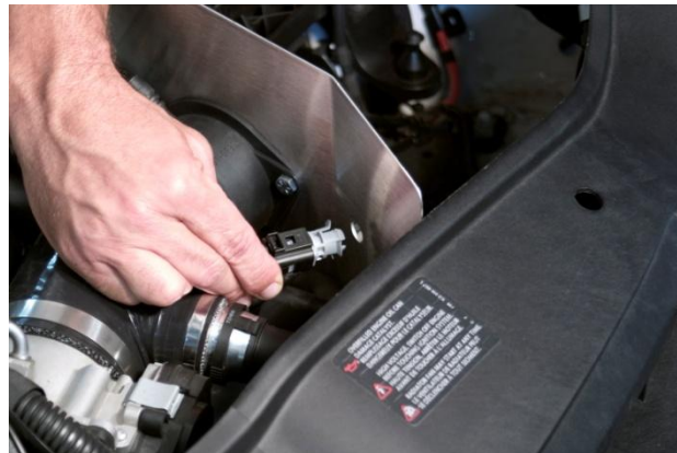
17. For vehicles equipped with air temp sensor, route wire under stainless steel bracket and from engine side, insert into mounting hole in stainless steel bracket.
