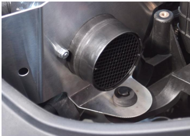
12. Insert MAF into silicone hose, and then push down stainless steel bracket onto pin mount just in front of the battery. Adjust bracket as necessary and make sure silicone hose is fully seated.
