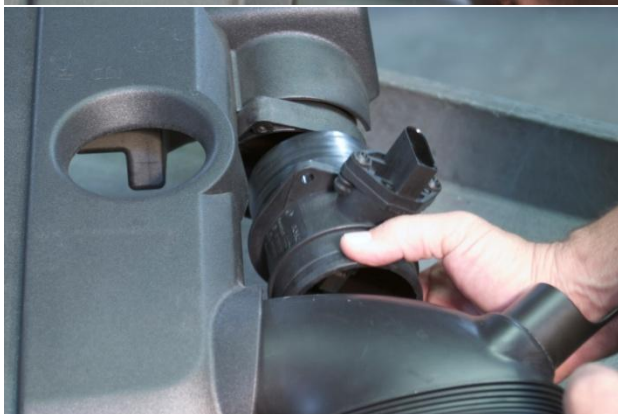
10. Remove (2) Phillips screws that mount the MAF to engine cover and separate.
