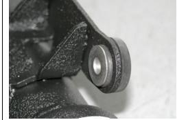
10. Remove rubber grommets and spacer sleeves from original pipe and install onto NEUSPEED pipe.
