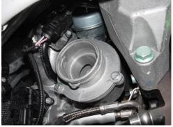
Unbolt original discharge adapter and separate adapter from turbocharger, (3) 10mm hex bolts. Note: Use caution not to damage O-ring. The O-ring is not available as a separate replacement
