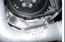
below crankshaft pulley, (2) T30 Torx.
