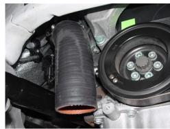
9. Install supplied silicone hose and clamp to turbocharger discharge adapter. Do not tighten clamp at this time.
