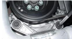
Unbolt aluminum pipe from engine just
