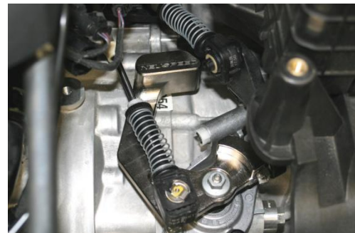
6. Grease guide rail on NEUSPEED® gear selector lever. Install selector lever by first installing guide rail in white plastic guide. Then match up splines on selector shaft – note wide alignment spline . Install lock nut and torque to 20 ft./lbs. Grease pin on gear selector lever and re-attach cable and retaining clip.
