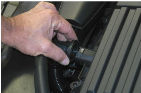
3. Squeeze collar and disconnect air pump hose from front side of air filter box lid if equipped.
