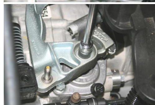
7. Remove clip on end of shifter cable and lift off. Unbolt gear selector lever from selector shaft using a 13mm socket – now remove lever (rock lever back and forth while pulling up).
