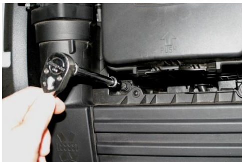
5. Using a 5mm hex key wrench, unbolt air filter box mount, located on back side.
