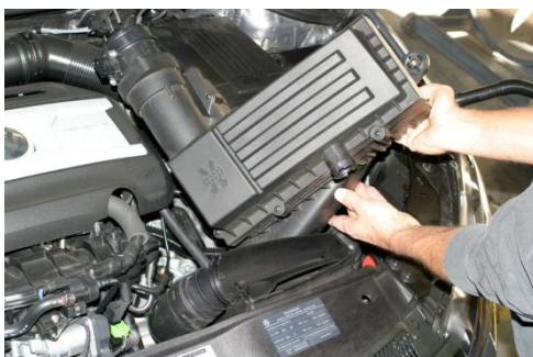
6. Lift off air filter box from rubber grommet mounts, then lift out left side first and rotate intake duct around small coolant hose to remove. Note drain tubing on bottom right side of air box.
