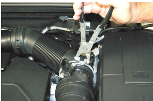
2. Disconnect air intake hose from MAF using spring clamp pliers.
