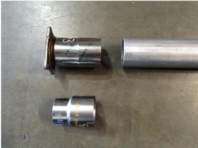
**Step 2.** Before installing your new system select the correct inlet adapter for your vehicles year. The larger adapter with the flange attached covers '01 - '05, the slip adapter covers '06 - '07. Attach the appropriate adapter by either bolting it to the vehicle outlet using the OEM fasteners or inserting the adapter into the slip clamp and loosely securing.
