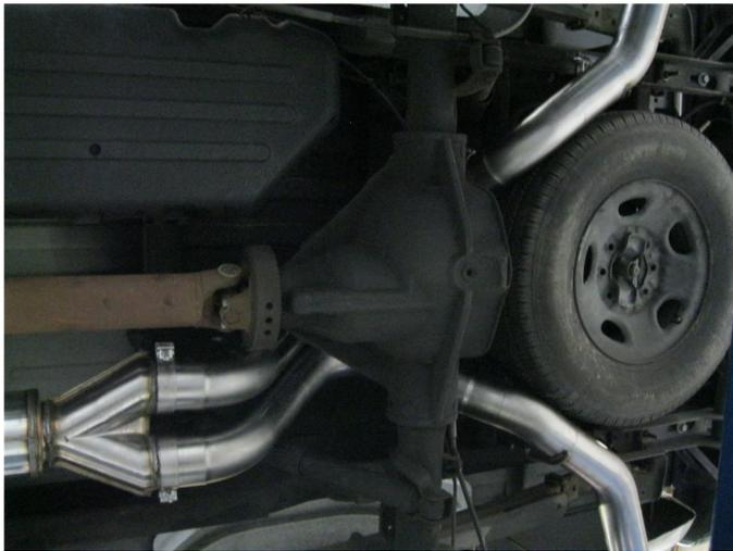
**Step 6.** Install both Over Axle Pipe Assemblies and the Tail Pipe Assemblies in a similar fashion.
