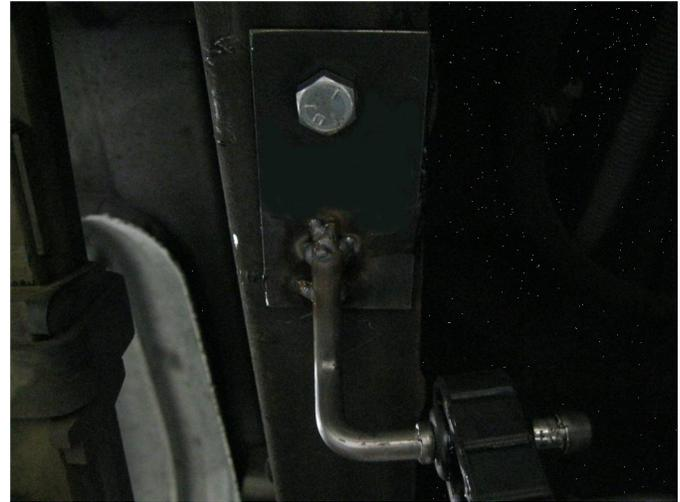
**Step 7.** For the Drivers Side Tail Pipe Assembly you will need to attach one of the supplied hangers. Bolt the supplied hanger bracket (shown) to the vehicles sub frame for year range '06 - '07. The threaded hanger is for year ranges '01 - '05. Both are mounted with the supplied hardware. Now engage the supplied hanger rubber to the newly mounted hanger and the welded hanger on the Tail Pipe Assembly.
