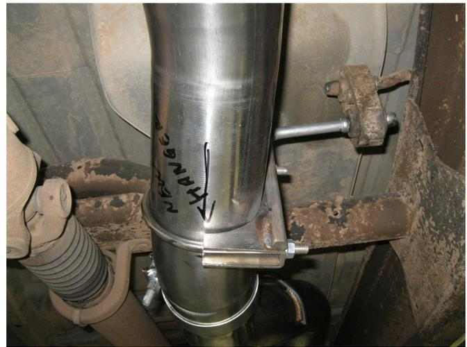
**Step 4.** For Short Bed models 13.00" needs to be cut from the outlet end on the Extension Pipe Assembly. Assemble and attach the U-Bolt Hanger assembly to the Extension Pipe Assembly as shown. There is a welded hanger on the pipe assembly that isn't used for Crew Cab, Short Bed versions of this truck. Loosely attach the Extension Pipe Assembly to the Mid Pipe Assembly using the supplied 4.00" Torca Clamp.
