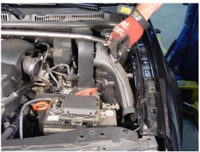
3. Remove side air duct by removing one (1) nut (10mm hex).
