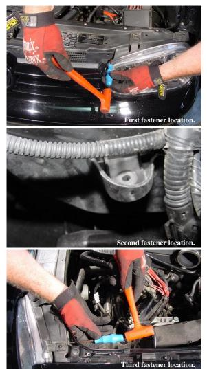
7. Remove the lower air duct housing by removing three (3) push fasteners. To release fastener, punch out center pin with a long reach screwdriver or punch and mallet. NOTE: First push fastener is located between driver's side headlight and grill. Second push fastener must be released from underneath the vehicle. Third fastener is located directly behind the driver's side low beam.
