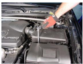
1. Remove entire factory air box by disconnecting Mass Air Flow meter (MAF) electrical connector, air pump connection (if applicable), and two (2) 10mm hex mounting bolts that hold air box to vehicle. Release MAF from rubber intake hose by squeezing spring clamp with needle nose pliers.
