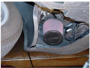
12. Install filter. **NOTE: Re-check tightness of filter clamp a week after installation.**
