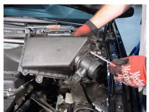
Remove MAF from air box lid by removing two
