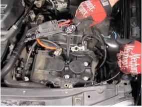
6. Remove two (2) bolts (10mm hex) securing fuse block to battery tray. Remove lower battery tray by removing four (4) bolts (10mm hex).
