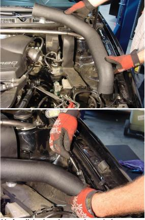
11. Install intake tube onto lower isolator mount using supplied M6 nylon lock nut (10mm). Then install tube onto upper fender mount using supplied washer and M6 nylon lock nut (10mm).
