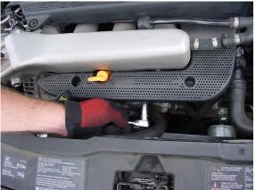
14. FOR AIR PUMP EQUIPPED CARS ONLY: To attach air pump tube to fitting, loosen clamp at the engine and slide tube through clamp for more slack. Now attach air pump tube to intake tube fitting making sure that it clips on completely. If necessary, apply a small amount of lubricant (i.e. WD-40) onto O-ring.
