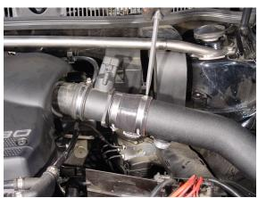
13. Slide two (2) hose clamps and reducer hose (2.0L & 1.8t) or straight hose (VR6) onto intake tube. Install MAF to factory intake hose (using factory spring clamp) and to hose on intake tube. Position and tighten remaining two (2) hose clamps.
