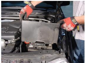
2. Remove battery box by removing one (1) bolt (10mm hex). Pull straight up to remove.
