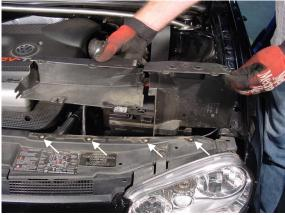
4. Remove four (4) Phillips screws securing upper air duct to core support and lift out.
