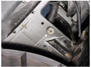
10. Install supplied rubber isolator into existing hole from underneath the vehicle using supplied washer and M6 nylon lock nut. **NOTE: Use hole closest to driver's side fender.**
