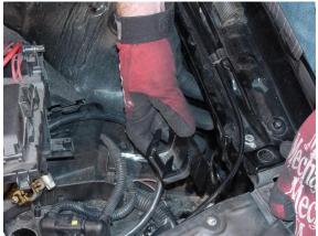
8. Pry off electrical connector bracket. This bracket is located against the lower, inside fender. Tuck wiring connector to side for now.
