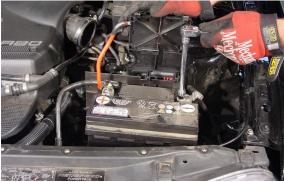
5. Disconnect and remove battery from vehicle – always remove negative post first. NOTE: Make sure that you have your factory radio's security code before removing the battery.
