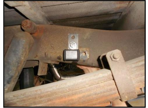
2) Locate the cross member at the front of the rear leaf spring, on the left side of this cross member, there will be a factory hole 9.00" in from the frame and  $\frac{3}{4}$ " up from the bottom, this hole location will need to be duplicated on the right side of the vehicle. Measure over 9.00" from the frame and  $\frac{3}{4}$ " up as shown in the photos below, use a center punch to make a mark and drill a  $\frac{5}{16}$ " hole on this mark.
