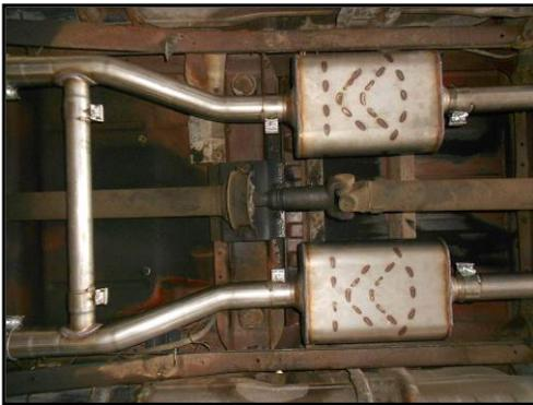
6) Take the right and left H-pipe assemblies, **86351** & **86352** and connect them together using cross over pipe **86360**. Place them up into position and connect the non-expanded ends into the muffler inlets. Make sure that they are fully seated. Support the front of the assembly with a stand. Place a provided 2" clamp at both of the cross over connections.
