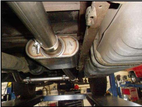
5) Place a supplied 2.5" clamp over the outlet of one of the **942545K** mufflers and slide onto the front of the right tailpipe, support the muffler with a stand and tighten the clamp enough to hold but still allow for adjustment. Repeat this step on the left side of the vehicle. Place another supplied 2.5" over the inlet of both mufflers.
