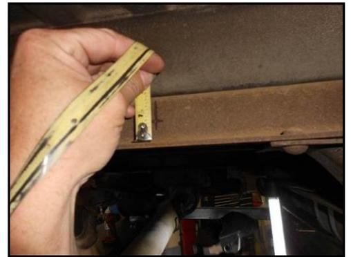
3) Remove the  $\frac{5}{16}$ " hardware from the parts kit, place a  $\frac{5}{16}$ " flat washer over the  $\frac{5}{16}$ " bolt and place thru the hole in the **211HA** hanger as shown below. Place the hanger into position with the bolt thru the frame; place a second  $\frac{5}{16}$ " flat washer over the bolt followed by a lock washer and nut. Make sure that the hangers are level and tighten securely. Place a **HA168** red exhaust isolator onto the end of each mount.
