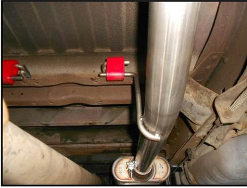
4) **Note:** For short bed model trucks, 14.00" will need to be trimmed from the front of each tailpipe. Place the right side tailpipe **#86353** up into position over the rear axle, slide the rear hanger on the pipe into the rubber mount on the frame and then connect the front hanger to the red exhaust mount. The red exhaust mount should hang straight up and down. Repeat this step on the left side of the vehicle with tailpipe **#86354**.
