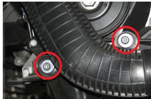
4. Unbolt plastic pipe from engine just below crankshaft pulley, (2) T30 Torx.
