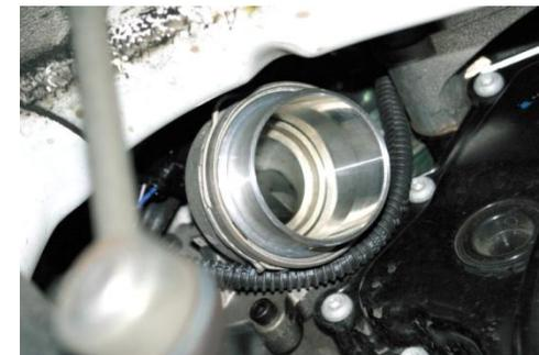
7. Lightly oil O-ring and install adapter into turbo making sure it locks into place.
