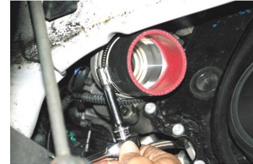
8. Install and tighten silicone hose to adapter using supplied #36 clamp.
