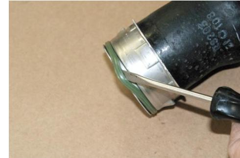
6. Carefully remove O-ring seal from original discharge hose and install onto NEUSPEED adapter.
