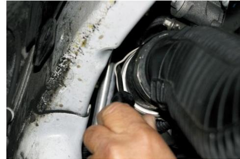
5. Pull-out clip to release rubber hose from turbo discharge.
