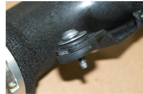
9. Pull-out mounting screws then rubber grommets from original pipe and install onto NEUSPEED pipe.
