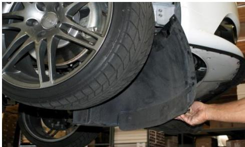
2. Undo the (8) T25 Torx screws to remove lower engine pan. Now remove the passenger side lower inner fender liner - there are (5) T25 Torx in the fender well and (2) T25 Torx on the bottom of the front bumper cap. **NOTE:** Some models may vary slightly.
