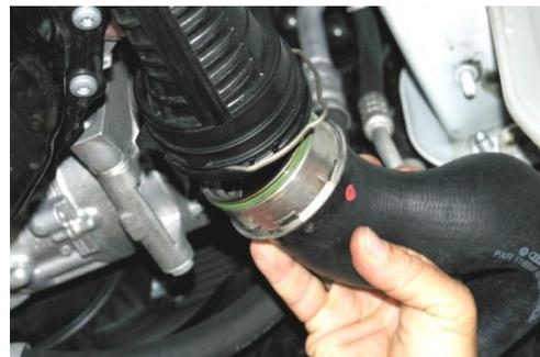
3. Use screwdriver to pull-out clip to release rubber intercooler hose from plastic pipe.
