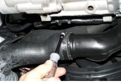
Loosen hose clamp using a 7mm nut driver or screwdriver at lower air charge pipe connection and disconnect from rubber hose.
