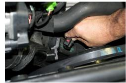
5. Disconnect electrical connection at boost sensor on air charge pipe.
