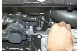
10. Use WD-40 or equivalent to lubricate inside of upper rubber hose and generously loosen hose clamp to ease pipe installation. Install *NEUSPEED* pipe from underneath and insert into upper rubber hose. Attach pipe mount to engine and tighten.
