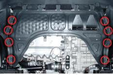
Raise the front of vehicle and support with jack stand(s) under lifting points. NEVER WORK ON A VEHICLE ONLY SUPPORTED BY A JACK. Remove lower engine splash pan, (8) T25 Torx screws. NOTE: GTI shown in picture, other models may vary.
