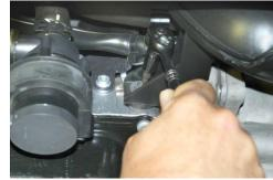
8. Unbolt lower air charge pipe mounting screw, T30 Torx. Pull-out pipe downward from underneath the vehicle to remove.
