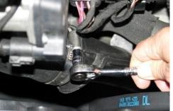
Loosen hose clamp with a 7mm socket or short screwdriver at top of plastic air charge pipe below throttle body.
