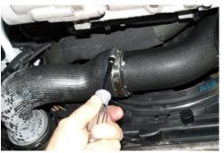
11. Use WD-40 or equivalent to lubricate inside of lower rubber hose and generously loosen hose clamp to ease pipe installation. Attach lower rubber hose to *NEUSPEED* pipe. Check alignment of *NEUSPEED* pipe and tighten lower hose clamp.
