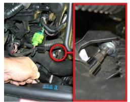
4. Unbolt upper air charge pipe mount using a 30 Torx.
