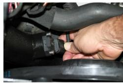
14. Reconnect electrical connection to pressure sensor. Double check complete installation.
