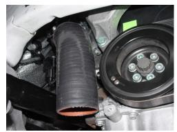
Install supplied silicone hose and clamp to turbocharger discharge adapter. Do not tighten clamp at this time.
