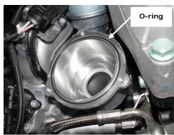
7. Make sure O-ring is properly seated in groove of turbocharger housing.
