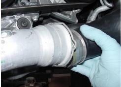
Use screwdriver to pull-out clip to release rubber intercooler hose from aluminum pipe.
