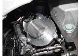
Install NEUSPEED billet discharge adapter using original bolts. Torque bolts to 4 – 5 ft. lbs.
