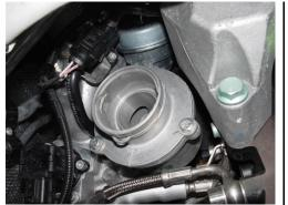
Unbolt original discharge adapter and separate adapter from turbocharger, (3) 10mm hex bolts. Note: Use caution not to damage O-ring. The O-ring is not available as a separate replacement part.
