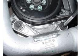
Unbolt aluminum pipe from engine just below crankshaft pulley, (2) T30 Torx.
