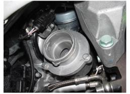
Unbolt original discharge adapter and separate adapter from turbocharger, (3) 10mm hex bolts. Note: Use caution not to damage O-ring. The O-ring is not available as a separate replacement
