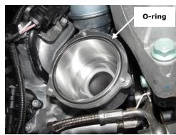
Make sure O-ring is properly seated in groove of turbocharger housing.
