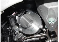
NEUSPEED billet discharge Install adapter using original bolts. Torque bolts to 4 - 5 ft. lbs.
