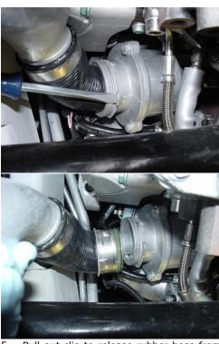
5. Pull-out clip to release rubber hose from turbo discharge.
