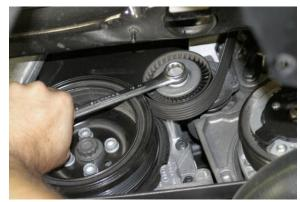
3. Using a 16mm wrench, rotate idler pulley center bolt upwards to release tension and remove belt. Now slowly release belt tensioner.
