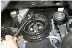
4. Use a 10mm Triple Square to loosen the (4) bolts securing pulley to crankshaft.
