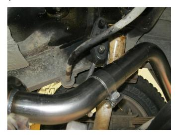
**Step 3.** Loosely attach the Tail Pipe Assembly using the supplied 2.50" clamp.
