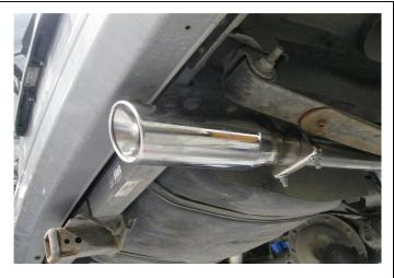
**Step 4.** Loosely secure the tip section of the Tail Pipe Assembly to the OEM hanger using the supplied 2.50" U-Bolt clamp.
