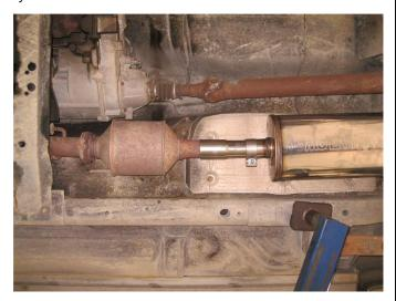
**Step 2.** Install the new system by attaching the new muffler assembly to the catalytic converter using the supplied 2.50" clamp and by locating the welded hanger to the rubber isolator. Be sure to align the locating notch in the muffler pipe with the indexing peg on the OEM system. Leave all clamps and fasteners loose for final adjustment of complete system.
