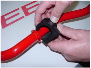
4. Apply silicone grease to the inside of supplied bushings and install on the inside of stop washer on *NEUSPEED* anti-roll bar.
