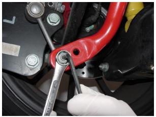
6. Attach end-links to *NEUSPEED* anti-roll bar using original nuts. **NOTE: The endlink to anti-roll bar bolt is easier to install with suspension loaded, put vehicle on ramps.** Torque to 40Nm (30 ftlbs). Forward hole is softer setting; rearward hole is stiffer setting (more oversteer).
