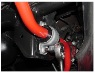
5. Install *NEUSPEED* anti-roll bar using original clamps and bolts to sub-frame. Torque bolts to 20Nm (15 ft-lbs).
