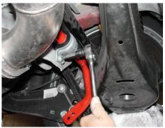
Install NEUSPEED anti-roll bar using original clamps and bolts to sub-frame. Torque bolts to 20Nm (15 ft-lbs).
