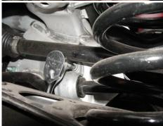
Remove four bushing clamp mounting bolts using a M10 Triple Square or 8mm hex key wrench. Now remove original anti-roll bar from vehicle. NOTE: To access upper clamp bolts, suspension must be compressed to raise drive axel.
