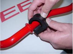
Apply silicone grease to the inside of supplied bushings and install on the inside of stop washer on NEUSPEED anti-roll bar.
