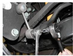
Disconnect end-links from original antiroll bar by securing stud with M6 Triple Square or 5mm hex key wrench and loosening nut with 16mm wrench.
