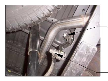
"STABILIZER LINK-TO-FRAME" BOLT TORQUE SHOULD BE 44 - 59ft-lbs.
