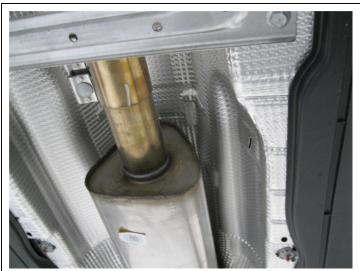
**Step 1.** Begin by loosening the factory clamp located just behind the catalytic converter. Working rearward extract the hangers from the rubber insulators (retain insulators as they will used in the installation of the new exhaust system). Remove the OEM system from the vehicle.
