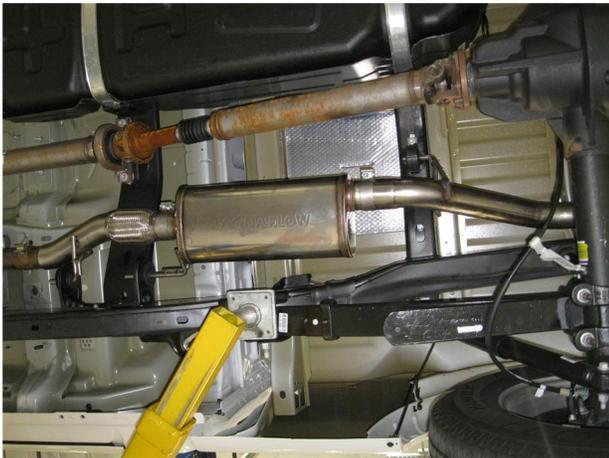
**Step 2.** To begin, fasten the Inlet Pipe Assembly to the catalytic converter using the OEM clamp assembly and by fitting the welded hanger into the OEM rubber insulator (Leave all clamps and fasteners loose for final adjustment of the complete system.) Install the Muffler to the Inlet Pipe Assembly using the supplied 3.00" clamp and fitting the hanger. Next install the Tailpipe Extension to the Muffler in the similar fashion using the supplied 3.00" clamp.
