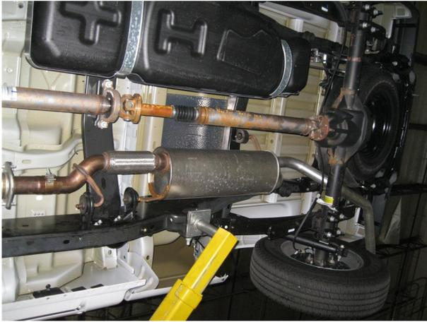
**Step 1.** To remove the OEM exhaust system, you will need to cut the pipe behind the muffler before it goes over the axle. You can then disengage the welded hangers from the OEM rubber insulators and remove the tailpipe. Unfasten the clamp attaching the OEM muffler inlet to the OEM catalytic converter. Do not damage or discard the OEM fasteners or rubber insulators, as they will be reused to mount the new system. Disengage the muffler hangers and remove the OEM exhaust from the vehicle.
