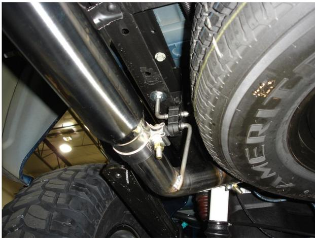
**Step 2.** Before installing your new system, to convert the vehicle to dual tips you must install the supplied threaded hanger into the driver side frame rail with the supplied fasteners as shown.
