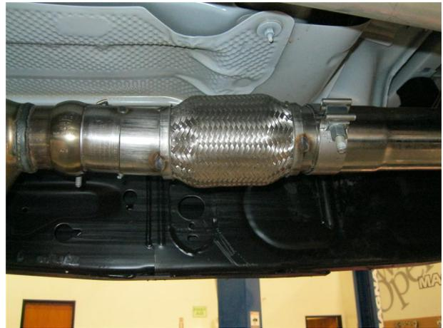
**Step 3.** Install the new Inlet Pipe Assembly at the ball flare using the OEM clamp. Leave all clamps and fasteners loose for final adjustment of the complete system.
