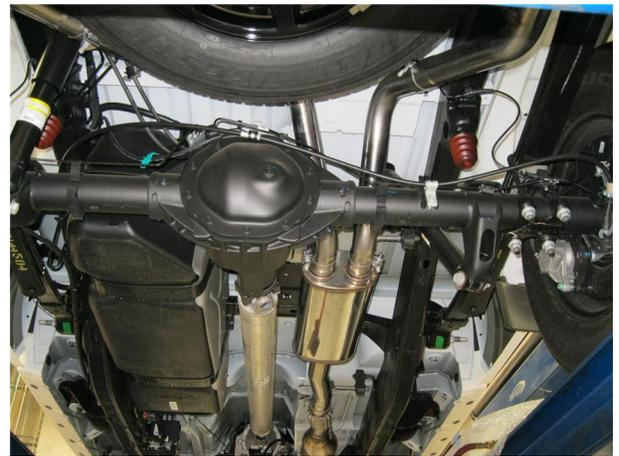
**Step 4.** Working front to rear install the remaining pieces of the MAGNAFLOW system, inserting hangers into rubber insulators and loosely installing supplied clamps. Adjustable tips are supplied to fit a variety of aftermarket bumpers and rollpans, once a position is decided for the tips it is recommended to have them welded into place.
