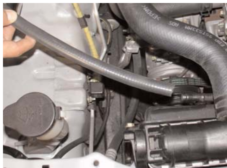
The 14"-10mm hose is pressed over the charcoal canister hard pipe.
