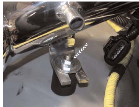
The flange nut and fender washer is screwed onto the vibra-mount stud. Do not over-tighten the flange nut at this point until the filter has been placed on the end.
