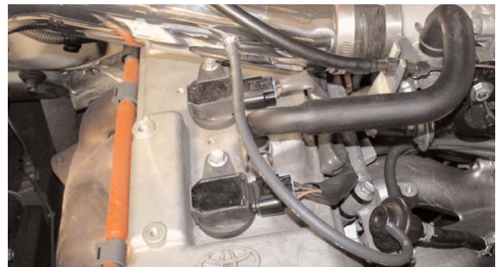
A good shot of the 4mm line connected to the pressure fuel regulator and the 3/16" intake port.
