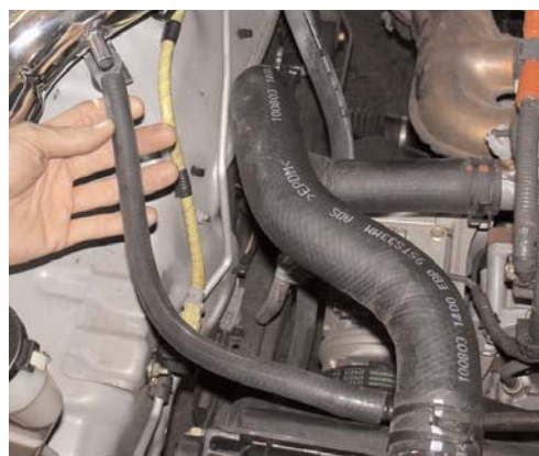
The 14"- 10mm vacuum hose is now pressed over the 1/2" intake port as shown above.
