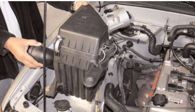
Remove the m6 bolts holding the air intake box to the fender well. Pull the air intake box out of the engine compartment.
