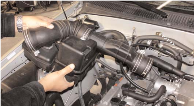
Loosen the clamps on the air intake box and the throttle body, then continue to remove the air intake duct as shown above.
