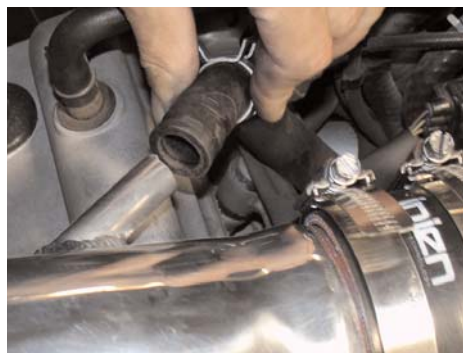
The stock crank case breather hose is reconnected to the 5/8" intake port located by the firewall.
