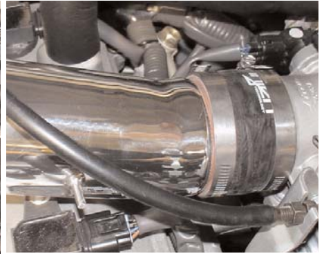
The intake is inserted into the throttle body hose and the intake bracket is lined up to the vibra-mount stud.
