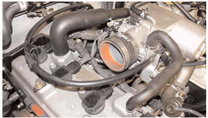
Press the 2 3/4" straight hose over the throttle body and use two .312 powerbands. At this point, you will only tighten the band on the throttle body side.
