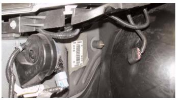
Take the vibra-mount and screw it into the pre-tapped 6mm hole. Screw the vibra-mount in until it completely bottoms out.
