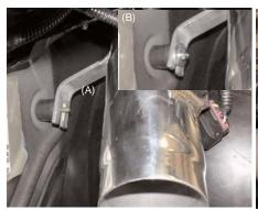
Once the top end has been pressed into the elbow continue to align the intake bracket to the vibramount stud(A). Use the 6mm nut and fender washer to fasten the intake in place (B).
