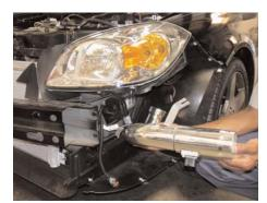
Carefully insert the 3" end of the intake into the corner bumper. Slip the 3" top end into the air duct opening.
