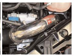
The 3" outlet on the end of the intake is now pressed into the silicone elbow as shown in this picture.
