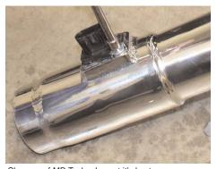
Close up of MR Technology at it's best. Once the mass air sensor is has been inserted into the adapter, use the 4mm button head screws to firmly secure the sensor in place.
