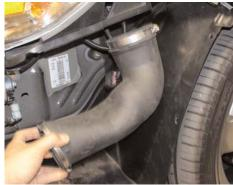
Remove the secondary air intake duct leading into the engine compartment.
