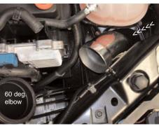
Top view of the intake inserted into the engine compartment before aligning it to the 60 degree elbow.
