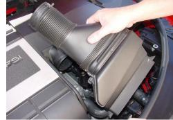
1 Remove the intake air duct: There are two T20 Torx screws that attach duct to the front core and a spring clamp at hose connection to the air filter box (engine cover).
