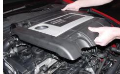
There are four rubber grommet mounts 4. holding air filter box (engine cover) to engine. Lift up one corner of air filter box at a time to detach.
