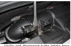
3. Unclip and disconnect turbo intake hose from air filter box.
