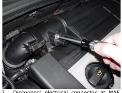
2. Disconnect electrical connector at MAF (Mass Air Flow) sensor and remove sensor mounting screws (T20 Torx), now pull out sensor.
