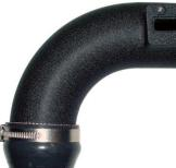
8. Install silicone hose onto turbo side of NEUSPEED intake pipe and tighten with #44 clamp supplied. NOTE: Screw clamp should be rotated toward passenger side of vehicle.
