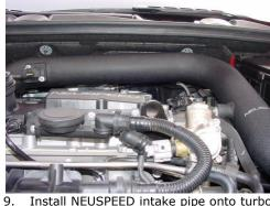
Install NEUSPEED intake pipe onto turbo inlet with #40 clamp supplied and attach rubber isolator mount to ear on end of cylinder head with M6x10mm screw. Intake pipe should be positioned at an upward angle toward brake fluid reservoir for engine torque clearance, now tighten hose clamp and M6 screw. NOTE: When tightening isolator mount, do not over tighten – rubber isolator should not have any twisting force applied to it.
