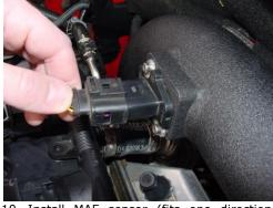
10. Install MAF sensor (fits one direction only) and tighten with two M4x8mm Philips head screws supplied. Attach electrical connector.
