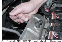
Install NEUSPEED heat shield: Unscrew the (2) rear mounts for factory air filter box (engine cover) by first removing the 10mm hex nuts located on bottom side of factory heat shield.
