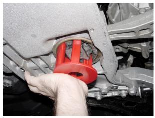
3. Use Silicone spray on urethane insert to ease installation, match up to rubber mount and push up until it bottoms out.
