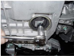
2. Unbolt the 21mm hex bolt from torque mount in aluminum sub-frame.
