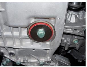
5. Install 3" stainless steel washer on to factory bolt and tighten into mount. Torque bolt to 74 ft. lbs.
