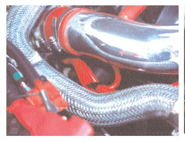
The 2 3/4" straight hose is attached to the throttle body using two clamps. The intake is then pressed into the straight hose as seen above. Do not tighten the clamps yet.
