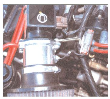
The cast adapter connects to the mass air flow sensor and the filter attaches to the adapter. The 1995-96 240sx has a sensor mount to bolt the air temperature control sensor using the stock
