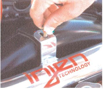
Use the stock screw to fasten the intake to the plastic fan cover, do not over tighten.
