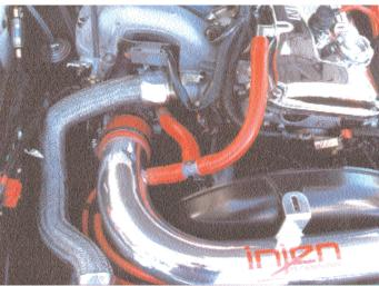
Use the three 15mm vacuum lines to connect to the ports on the throttle body and the valve cover as seen above. Use the plastic T-fitting to connect all lines to the 5/8" nipple on the intake. The 8"- 3mm vacuum line replaces the stock line that is underneath the intake near the throttle body.
