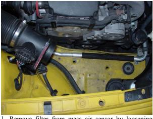
1. Remove filter from mass air sensor by loosening hose clamp and discard.
