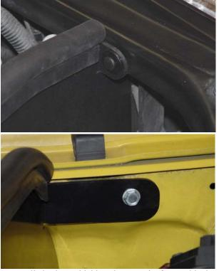
5. Install the heat shield and secure in front with the supplied push fastener and at the side with the supplied sheet metal screw as shown.
