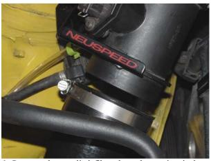
6. Pass newly supplied filter through opening in heat shield. Rotate filter until end of filter is parallel with mass air sensor. Slide filter onto sensor and secure hose clamp. NOTE: Check tightness of clamp in one week.
