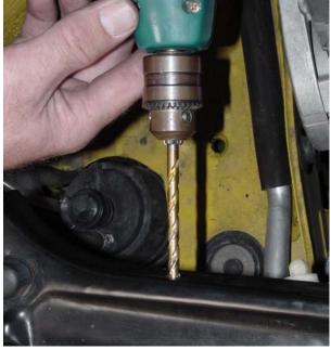
4. Install heat shield and using the front mounting tab hole as a guide, mark the radiator support. Remove the shield and drill a  $\varnothing$   $\frac{1}{4}$ " hole through the radiator support.
