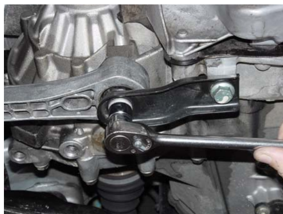
10. Install front bolts (16mm hex) and torque to 30 ft-lb + 90° (1/4 turn)
