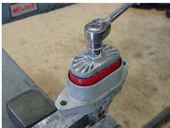
8. Install plate and secure isolator assembly with bolt. Torque to 20 ft-lb.
