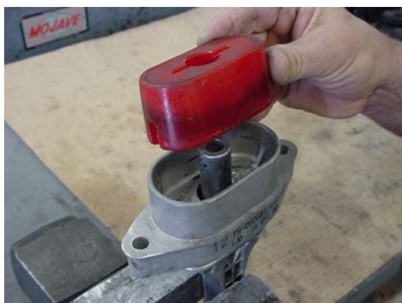
7. Install thick urethane isolator into mount in orientation shown.
