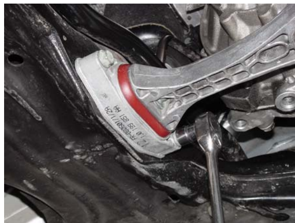
9. Position mount in cross member and install two bolts (13mm Hex). Torque to 15 ft-lb + 90° (1/4 turn)
