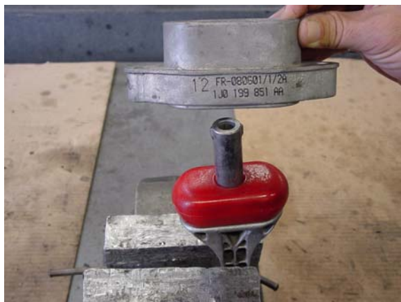
6. Install mount over isolator in orientation shown.
