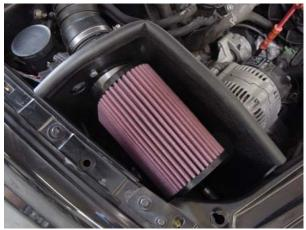
6. Mount mass air sensor to heat shield using existing <sup>1</sup>/<sub>4</sub>" bolts and lock nuts. Install air filter on mass air sensor and tighten hose clamp. **NOTE: Check tightness of clamp in one week**.
