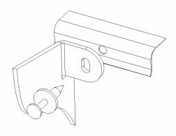
3. Due to slight variations in vehicle geometry (see illustration above), it is necessary to drill the radiator support to properly mount the heat shield. Pull the heat shield forward (towards the front of the car) until the mounting tab contacts the radiator support. Using the front mounting tab hole (slotted) as a guide, mark and center punch the radiator support.
