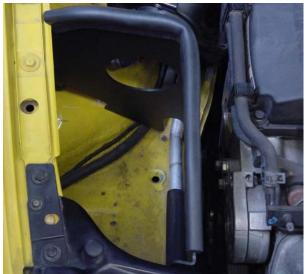
2. Insert lower front portion of the shield under the radiator support and slide bottom edge of shield into slot between AC condenser line and chassis seam. Rotate rear portion of shield down and into position, making sure any hoses and/or electrical lines are routed through cut outs.
