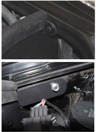
5. Install the heat shield and secure in front with the supplied push fastener and at the side with the supplied sheet metal screw as shown.
