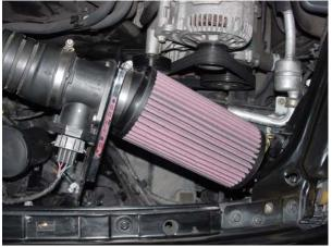
1. Remove filter from mass air sensor by loosening hose clamp and discard.
