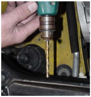
4. Remove the head shield and drill a  $\emptyset$  <sup>1</sup>/<sub>4</sub>" hole through the radiator support.
