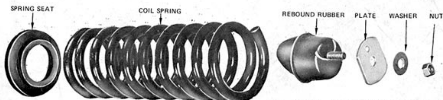
Coil Spring and Rebound Rubber Removed from Rear Suspension Arm. (Sedan).
