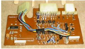
There are two small plastic retaining clip which holds the circuit board inside the beige box. Sliding a screwdriver underneath one and then the other will release the circuit board. Slide it forward. The solder joints you are interested in are on the underside of the circuit board.
