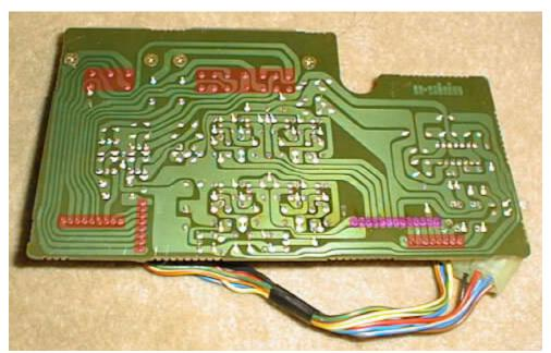
Make sure that your solder joints are nice and shiny (i.e. heat the metal, not the solder, etc.), otherwise you'll be doing this all again in the near future! Slide it back into the beige box when you're done.
